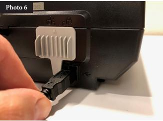
c. Remove the USB cable from the zipper pocket of the suitcase (see Photo 5) and plug it into the back of the scanner (see Photo 6). Slide the grey scanner lock to the left if it is in the way.
